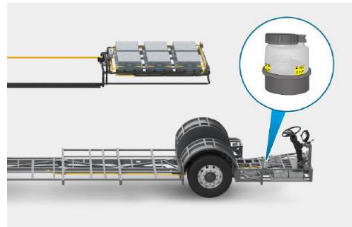
Schematic diagram of position of steering fluid reservoir
