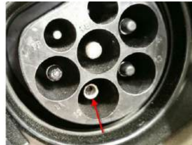
Contact prevention cap fall-off
